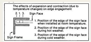
Adequate edge engagement is also important to prevent the face from disengaging or dropping out in high winds. See the following section.
